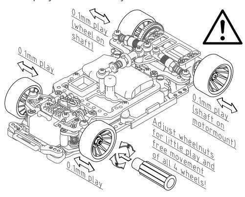
**STEP 5.2.3:** Check rear wheels for easy opposite side rotation of differential:
