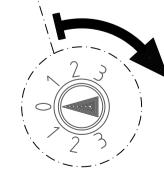
... TURN THrottle TRIM knob SLIGHTLY CLOCKWISE until car stopps completely & adjust about 1mm gap from neutral position for forward & backward function.
