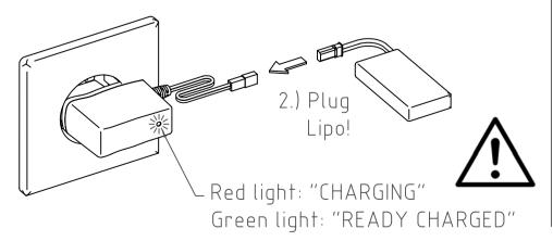
**STEP 5.1.3:** After light on charger has changed to green unplug the Lipo battery immediately from the charger. Then unplugg charger from the socket:
