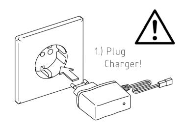
**STEP 5.1.2:** After plugging Charger to the socket, plug Lipo Battery to the Charger. (RED LIGHT on charger: "CHARGING"; GREEN LIGHT: "READY CHARGED"):
