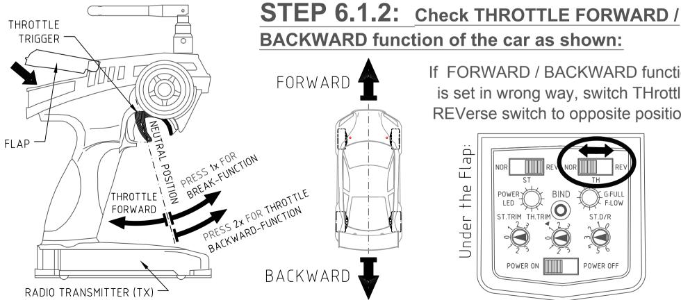
If FORWARD / BACKWARD function is set in wrong way, switch THrottle REVerse switch to opposite position:
