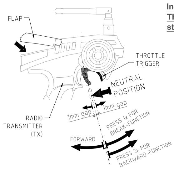
In NEUTRAL POSITION of the THROTTLE TRIGGER the car has to stand still without any movement!
